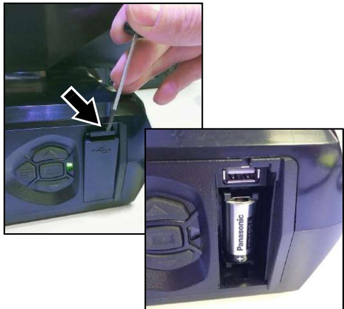
Figure 9: Compartiment de pile
