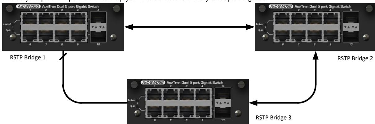
Fig 6: A simple loop network with RSTP
