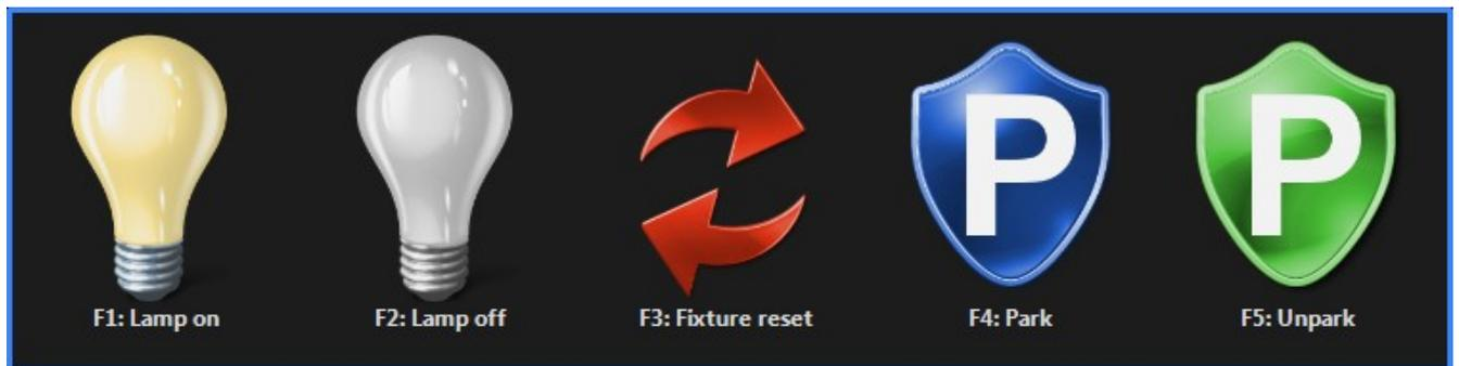
**Note: When using the Lamp ON and OFF commands, the console will "stagger" DMX output randomly so that the command is not received by all the fixtures simultaneously.**
