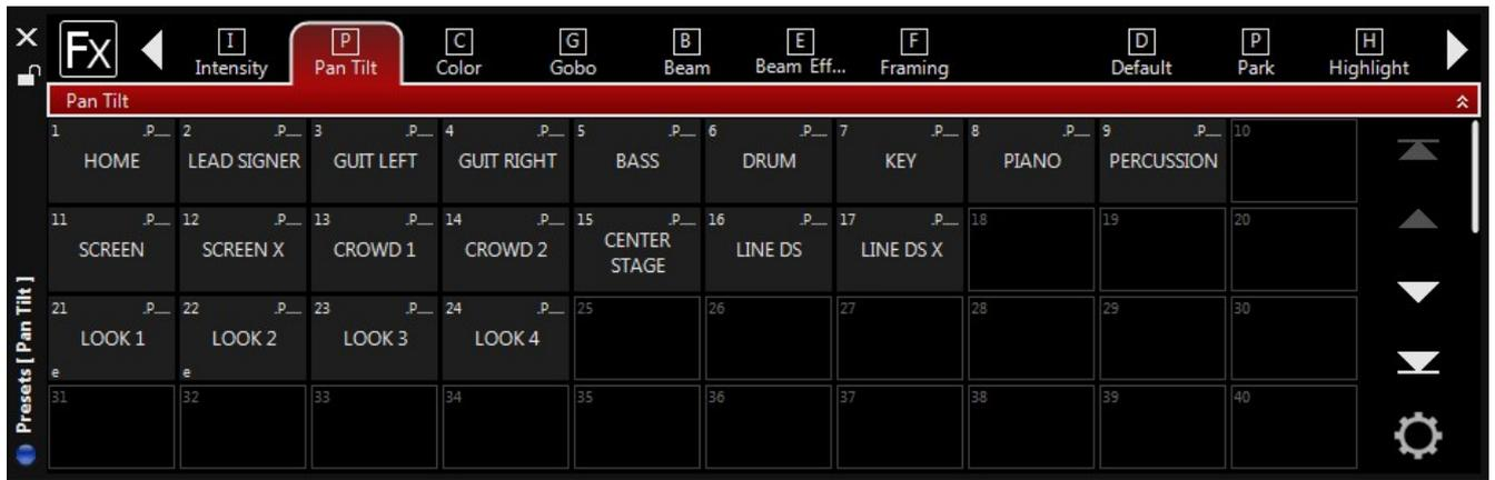
Activate the preset screen by pressing the view button directly over the “Programmer Preset” label on the playback touch screen. At the top of the preset screen are 10 buttons with the following functions.
