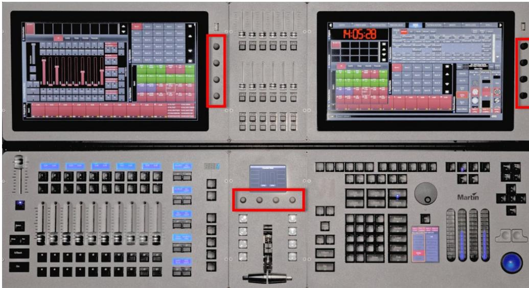
The Fast Dial encoders on the M6 console are user assignable to any parameter currently available on the belts.
