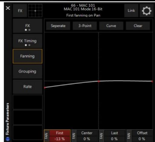
As you can see, in the Mirror example, the First and Last attributes are at +/-13% even though only the First fan attribute was adjusted. This is because as the First fan attribute was altered to -13%, the Last fan attribute mirrored it and moved to +13%. In the Separate example the First fan attribute is at -13% but the Last fan attribute has remained at 0%.
