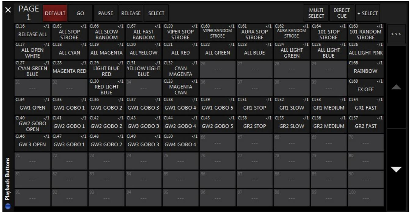
At the top of the screen you can see the controls for the playback buttons. The up and down arrows at the right side increment and decrement through the 99 available Playback Button pages. Pressing the “>>>” directly above the “Up” button, opens a direct select option for rapidly jumping to the desired page.
