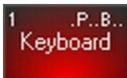
The letters “P” and “B” indicate that there is both Pan Tilt and Beam information in the preset. You’ll also note that the field is red. This indicates that this is the last selected/played preset on the page. The different shades of gray indicate whether or not a selected fixture is contained within a preset. Presets displayed in dark gray contain at least one of the currently selected fixtures, light gray presets contain none.
