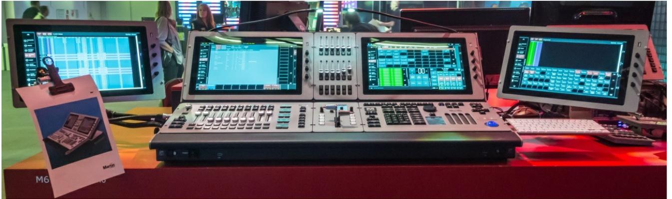
M6 allows to attach VESA 100mm compatible screens to the outside of the desk, including the two screen modules.
