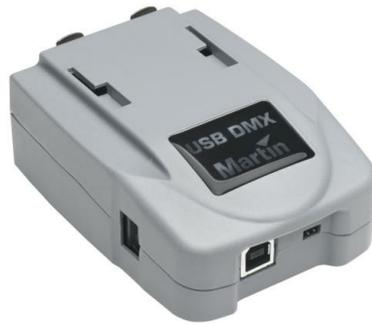
The USB DUO DMX box, allows a user to add 2 extra physical DMX outputs to any M-Series system. The box itself doesn't hold any additional licenses for extra universes, it only provides the physical 5 pin outputs. The box can be configured to provide two extra outputs or two extra inputs or any combination of Input/Output. See [USB2DMX section](#) in regards to configuring connected USB DUO DMX boxes.
