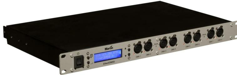
Ether2DMX8 is a highly capable DMX router and much more! As a DMX router, it translates Art-Net protocol into DMX in/out universes but can also be used as a DMX merger, DMX splitter hub, fail safe device, cue playback, and DMX viewer monitor. As an extension for the M1 and M2GO console it provides 8 additional DMX ports and includes the required DMX license. When connected to a standalone PC, the Ether2DMX8 also becomes the license key for M-PC and provides 8 DMX Universes.
