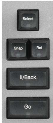
The Main Go and Main II/Back (pause/back) buttons are convenient, fast-access buttons for fading the next cue and pausing/fading the previous cue in the cue list designated as the *main* cue list. If no cue list is designated “as main”, then the Main II/Back and Go buttons control the *selected* cue list.
