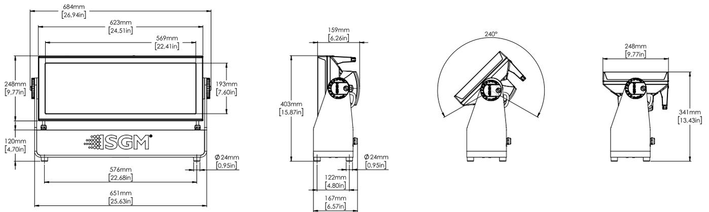
All dimensions in millimeters and inches. Drawing not to scale.
