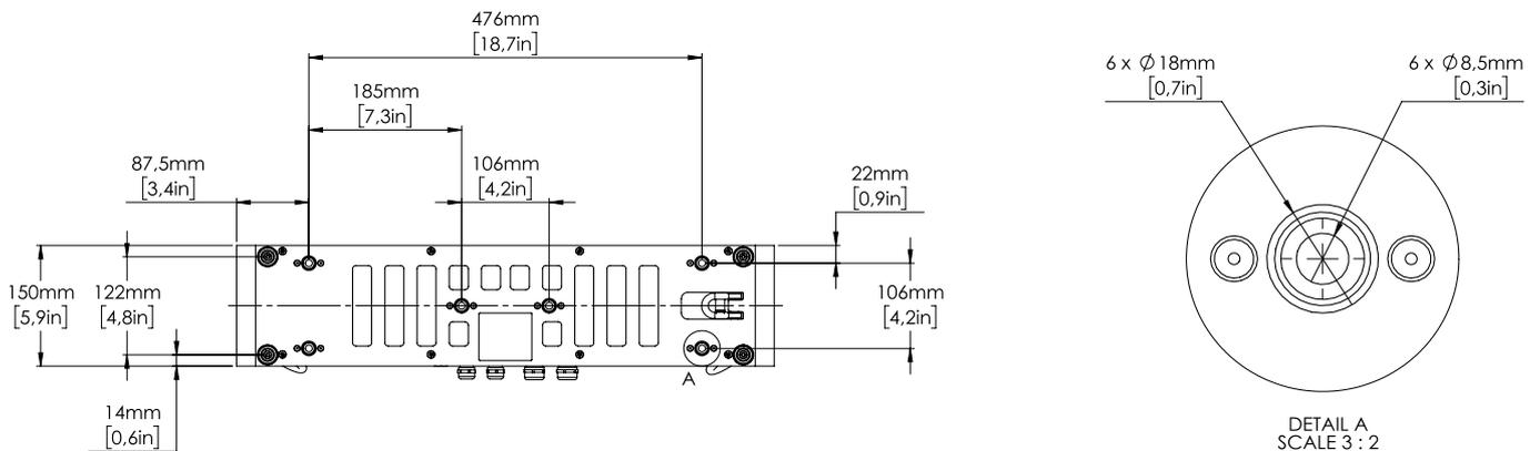
Figure 18: P-10 POI base with dimensions
