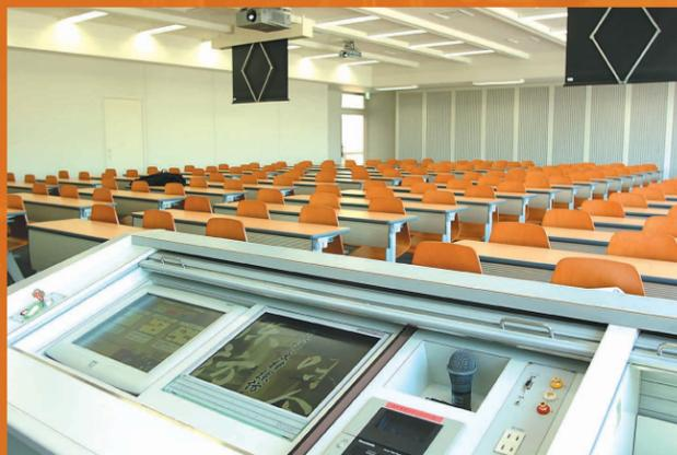
This 180-capacity classroom is also on the 1st floor. The equipment rack and control console can be seen at the front of the room to the left. The movable console includes a cassette player and other facilities for the convenience of the lecturer. A 120-inch main screen and two 60-inch sub-screens are provided for visual presentations.
